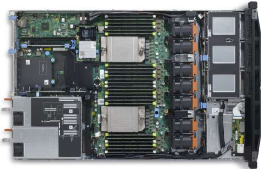
Figure 5. Eight-drive bay chassis internal view
