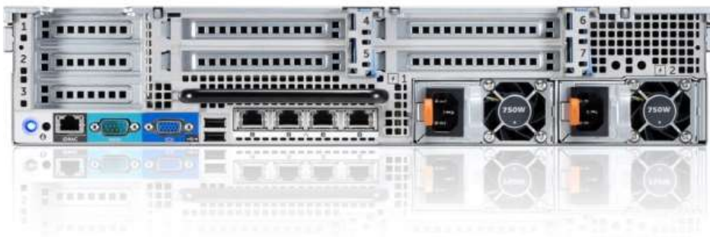
Figure 5. R720 back view
