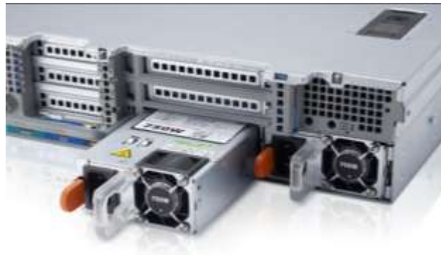
Figure 8. 750W power supply unit
